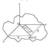
Moment of inertia about *x*-axis,  $I_x = mx^2$ Moment of inertia about *y*-axis,  $I_y = my^2$
