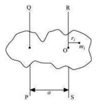
Suppose a rigid body is made up of *n* particles, having masses  $m_1$ ,  $m_2$ ,  $m_3$ , ...,  $m_n$ , at perpendicular distances  $r_1$ ,  $r_2$ ,  $r_3$ , ...,  $r_n$  respectively from the centre of mass O of the rigid body.
