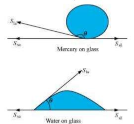
$S_{la}$ ,  $S_{sa}$ , and  $S_{sl}$  are the respective interfacial tensions between the liquid-air, solid-air, and solid-liquid interfaces. At the line of contact, the surface forces between the three
