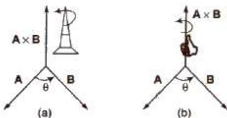
**(i) Right Hand Screw Rule** Rotate a right handed screw from first vector ( $\mathbf{A}$ ) towards second vector ( $\mathbf{B}$ ). The direction in which the right handed screw moves gives the direction of vector ( $\mathbf{C}$ ).
