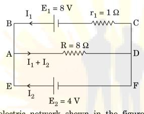
In the electric network shown in the figure, use Kirchhoff's rules to calculate the power consumed by the resistance  $R = 8 \Omega$ .
