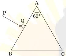
A ray PQ is incident normally on the face AB of a triangular prism of refracting angle of 60°, made of a transparent material of refractive index  $2/\sqrt{3}$ , as shown in the figure. Trace the path of the ray as it passes through the prism. Also calculate the angle of emergence and angle of deviation.
